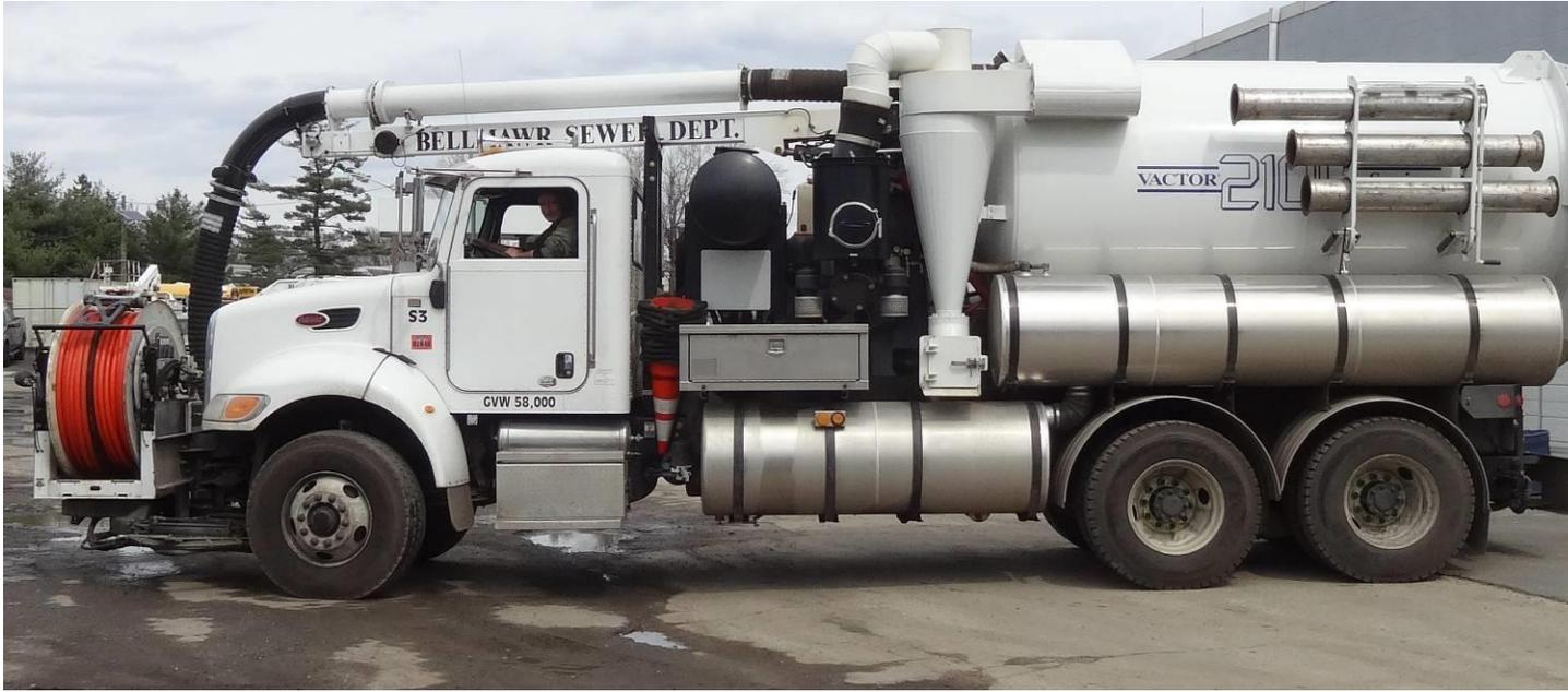
The sewer Jet/Vac is a specialized vehicle that uses highly pressurized water to flush and clean sewer mains and collects debris by a high velocity vacuum system. If while a maintenance crew is performing main line cleaning in your neighborhood and you experience disrupted sewer service, strange noises coming from your pipes, or water splashing from your toilet, please do not hesitate to contact the Sewer Department at 856-931-1111 so that we can rectify any disruption.
